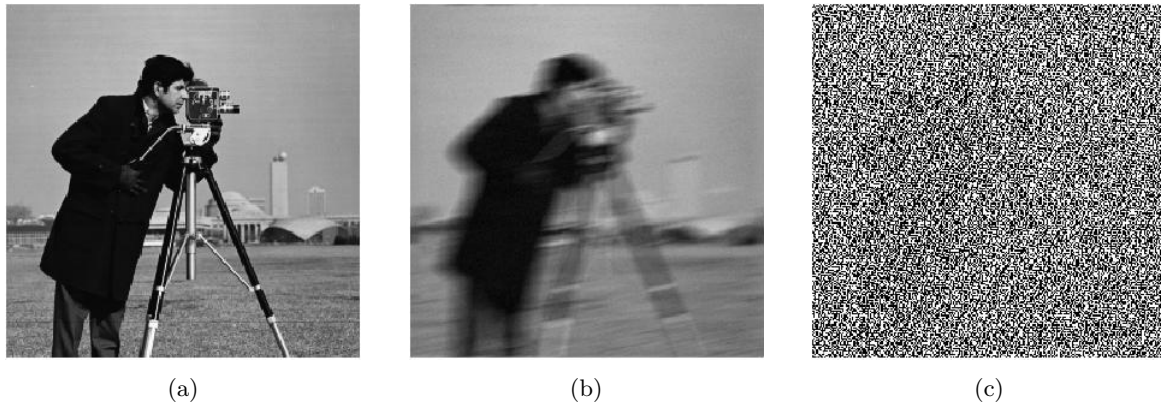
Figure 1: Naive Method: (a)original image ,(b) image degraded by a motion blur and noise by an additive Gaussian noise of variance \sigma = 0.0001 ,(c) restored image with the equation (3)
